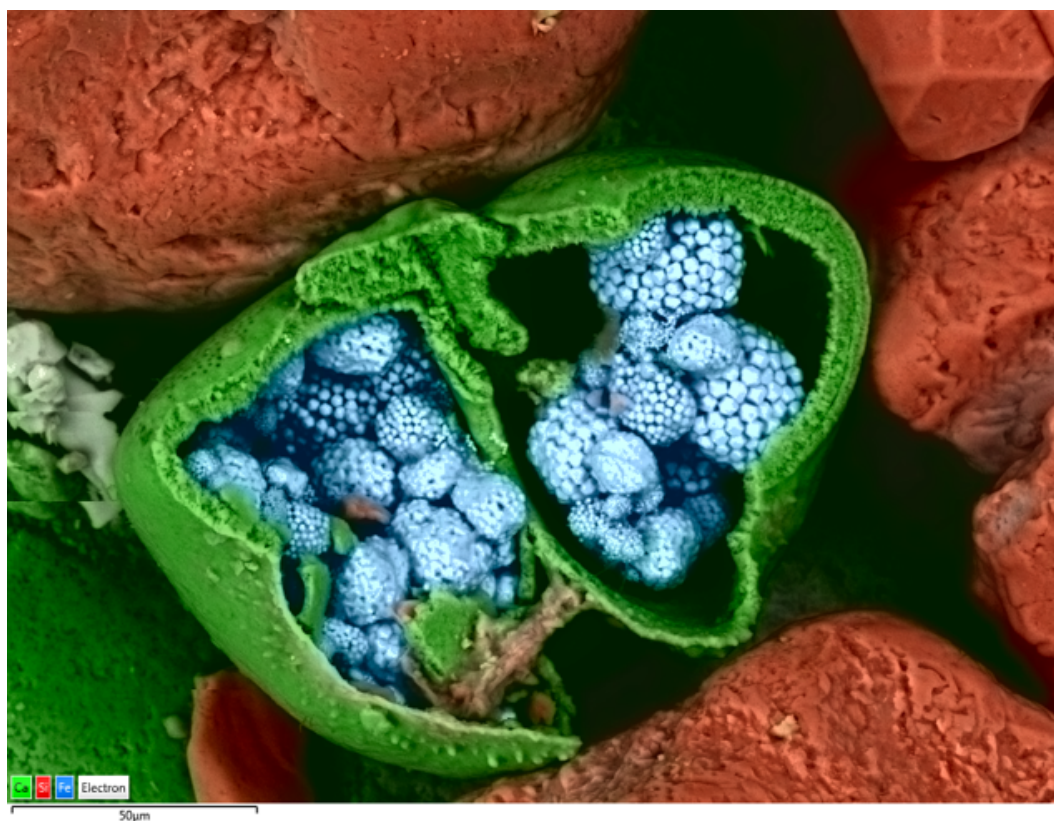
Figure 1 : Analysis of Micro-organism in seashell with BEX – Unity (20kV 50Pa 600X 15s)
